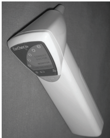
Fig. 1. Photograph of EarCheck® spectral gradient acoustic reflectometry instrument (MDI Instruments Inc, Woburn, MA, USA) used in this study.
