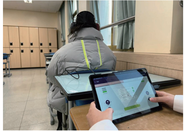
Fig. 2. Demonstration of hearing screening using easyTone at high school in Seoul. The participant is seated in a quiet classroom and wears earphones connected to a tablet device. The screening follows a fixed sequence of frequencies (500, 1000, 2000, and 4000 Hz) for both ears. When a tone is heard, the participant raises their hand to indicate detection. The examiner monitors ambient noise levels via the device and provides instructions as needed. This setup reflects the actual procedure used in school-based hearing screenings.
