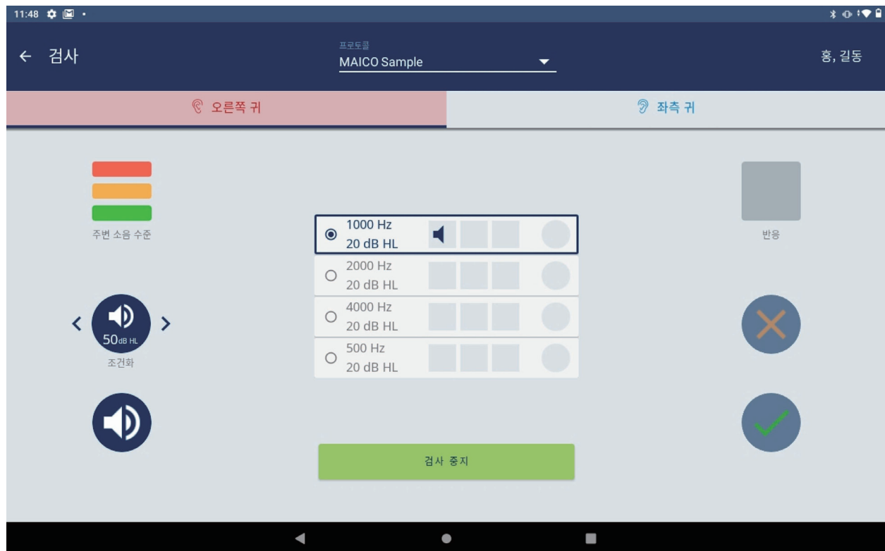
Fig. 1. Screenshot example of the easyTone screening interface. The interface displays selectable test frequencies, real-time ambient noise indicators (green, orange, and red), and user-friendly controls.
